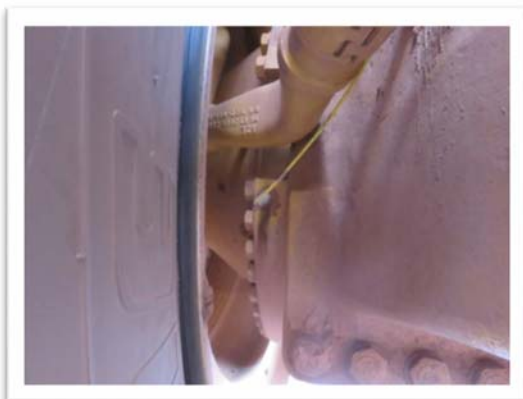
Sensor installed on the POS4 inner hub box inside the driver cabin
