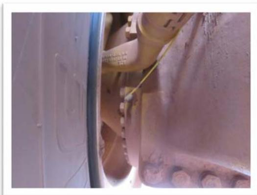
Sensor installed on the POS4 inner hub box inside the driver cabin
