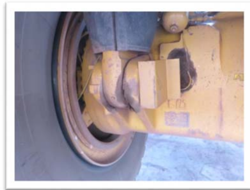
Sensor installed on the POS3 wheel hub
