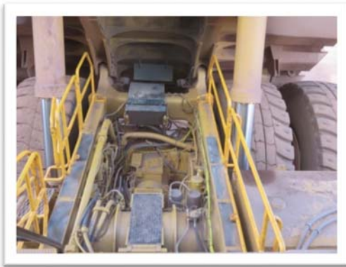
Sensors installed on the LHS and RHS of the differential
