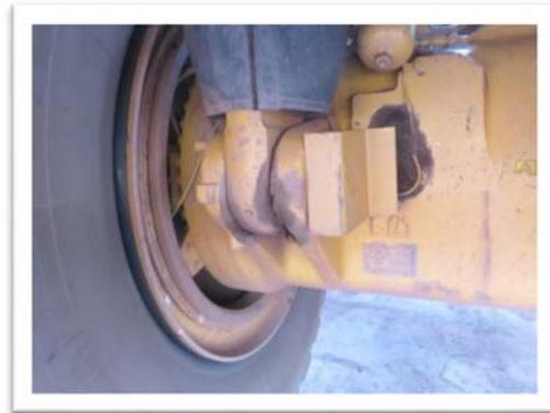
Sensor installed on the POS3 wheel hub
